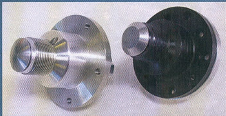
The Hollywood Hot Rods one-piece knockoff hub (left) is built to replace the knock-off adapter from PS Engineering that is matched with the hub that comes with So-Cal Speed Shop's outstanding Buick-style front brake system.
