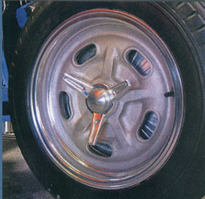
Buick finned drums with Wilwood disc rotors, lugless kidney bean wheels, bias-ply dirt track rubber, and three-pronged knock-offs; the unseen one-piece knock-off hubs from Hollywood Hot Rods are the piece that pulls together this whole cool combination.
